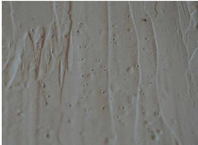
Figure 60: Bubbles in Flügger sample 13 after application.
