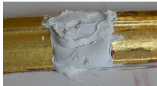
Figure 65: Modostuc fill on board
