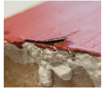
Figure 38: Area of lifting on Klucel G sample
