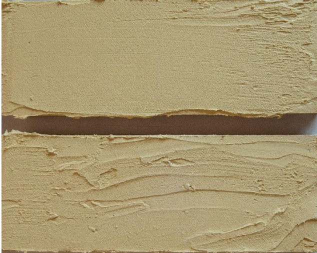
Figure 61: Ronseal samples before sanding showing texture of the material.
