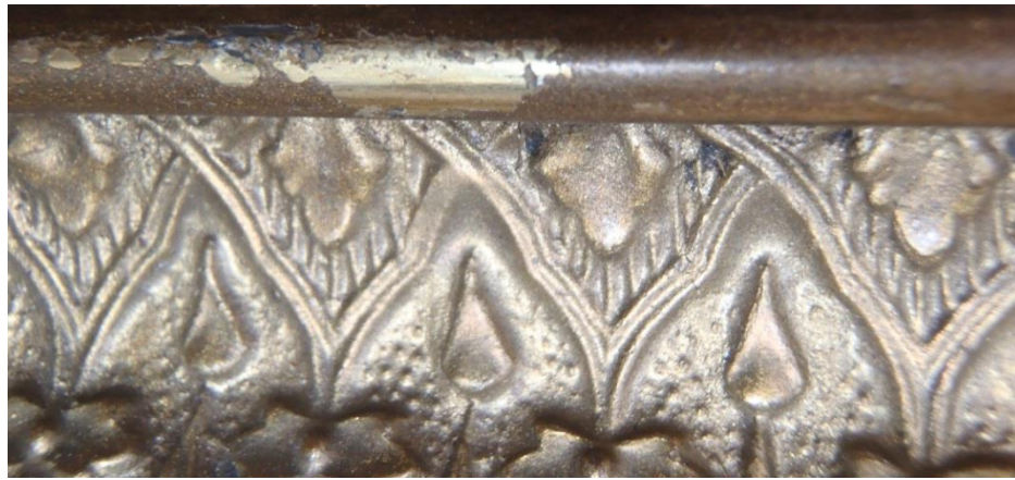
Figure 6: Bronze paint thickly applied over the surface of the frame. Original gilding can be seen in the upper left half of the image where the paint has flaked off. Image by author, personal collection.
