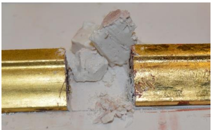
Figure 82: Modostuc fill after removal
