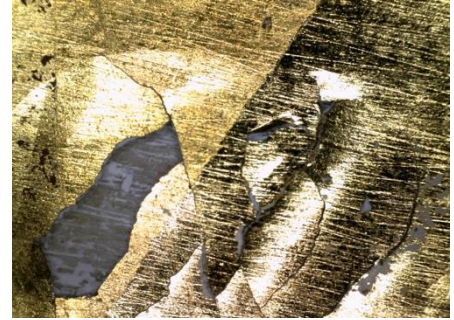
Figure 33: Cracking during burnishing on the B-98 sample. 50x magnification.
