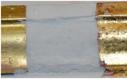
Figure 73: Modostuc fill after carving
