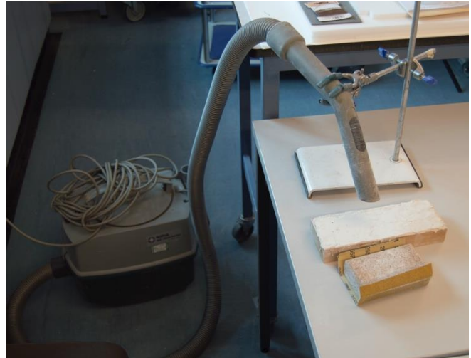
Figure 17: Nilfisk museum vac dust removal setup. A stronger shop vac is recommended for future tests as sanding produced a large amount of dust. Additionally, a particle dust mask is recommended.
