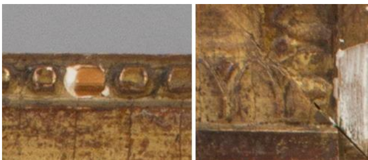
Figure 5: Damage to gilded frame 19590309_fr where gesso has been lost. Damage on right most likely caused by fluctuation of substrate at the mitred joint. Images courtesy of The Frick Collection.
