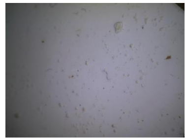
Figure 20: PVOH silicone mould surface at 20x magnification
