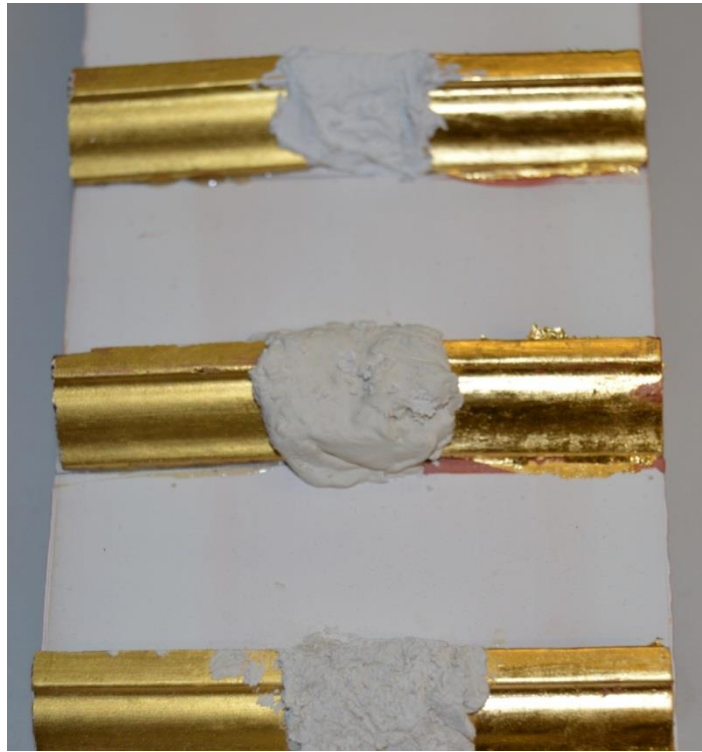
Figure 16: Sample board with fill samples placed. Water gilding is on the right side, and oil is on the left.
