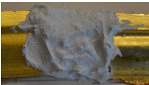
Figure 64: Lascaux Gesso fill on board
