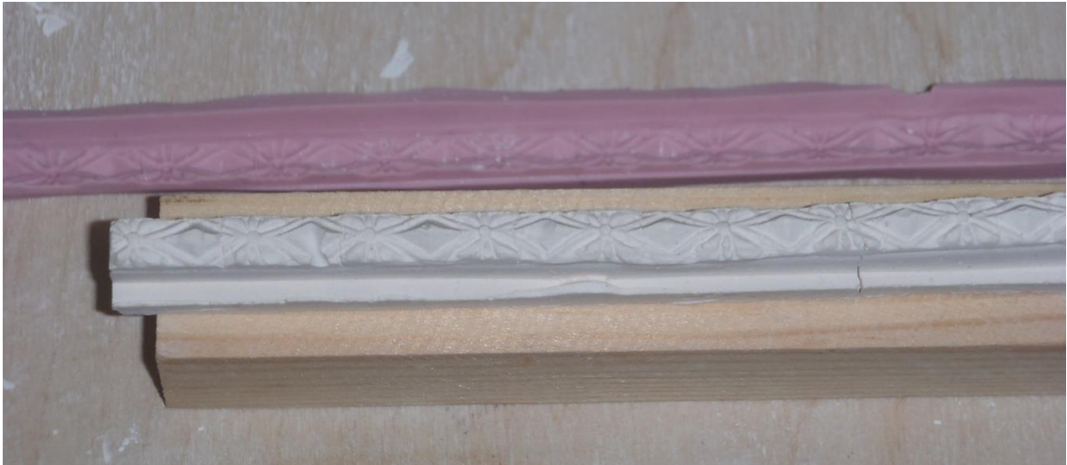
Figure 15: Dental mould and plaster cast of the decorative moulding. The cast was used to create a larger and sturdier mould for the actual tests.
