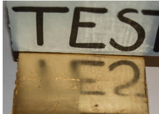
Figure 49: Lascaux Gesso burnish test. Softer burnish but better surface.
