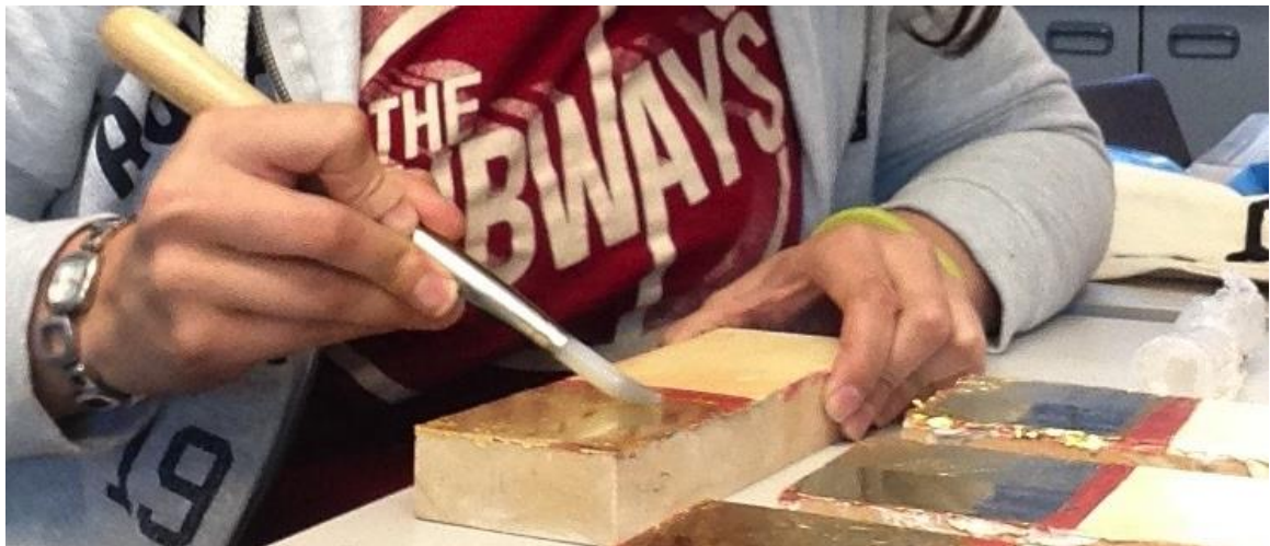
Figure 1: Burnishing of the water gilded samples using an agate burnisher. To the right are burnished samples with the reflective surface on the lower half of the squares. (Photo taken by author).
