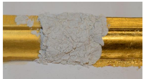
Figure 66: Crazing on the B-72 fill
