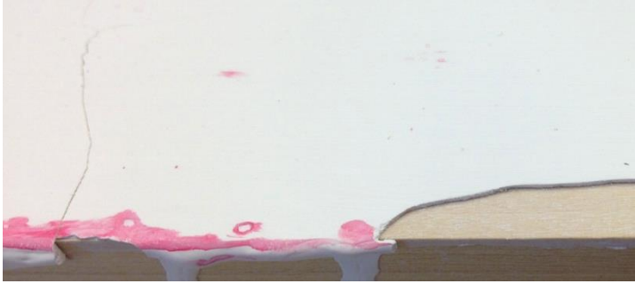
Figure 22: Cracking and lost areas on a B-98 sample
