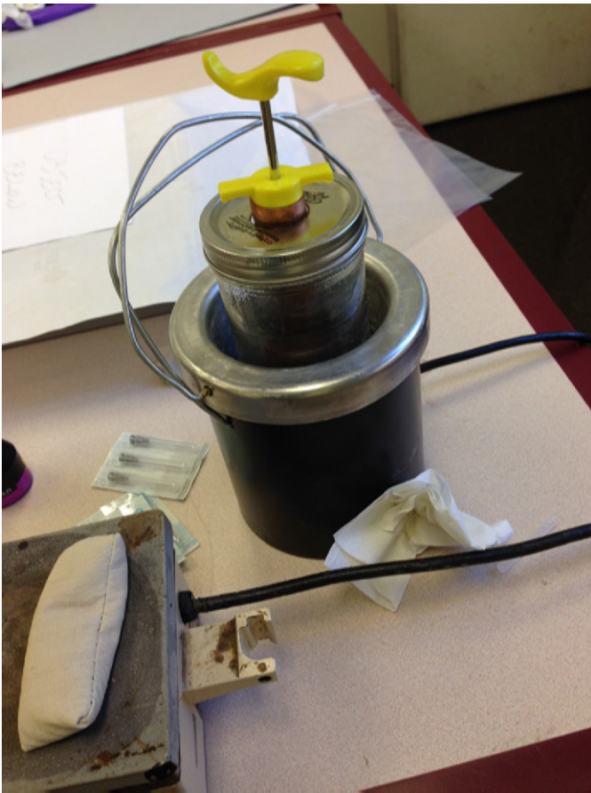
Fig. 6. Bain marie made of a modified mason jar with a copper tube set into the center of the lid. The mason jar was filled with water then placed into water in a standard glue pot. Courtesy of the Winterthur Museum.
