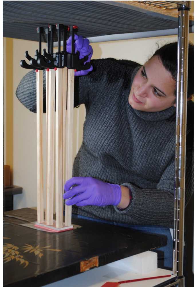
Fig. 7. Author Liz Peirce clamping using the Shimbari table. Courtesy of the Winterthur Museum.
